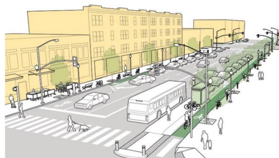
Figure 109 : Transit Oriented Development Facilities - Pedestrian Crossing, Segregated Lanes, Lane Markings, Bike Lanes
